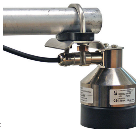
The 19517's bracket mounts directly to a crossarm. Two screws are used to attach the SR50A to the 19517 bracket.
